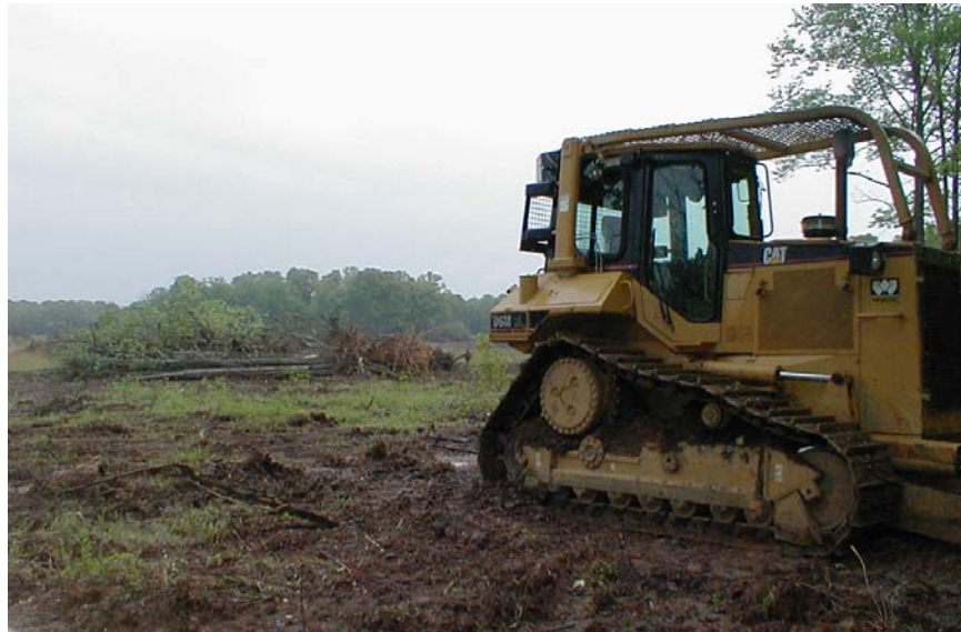
Figure 7. Dozer work to reclaim fields may cost $700 or more per acre.
